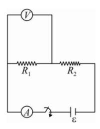
A. voltmeter reading is lesser than  $\frac{\varepsilon R_1}{R_1 + R_2}$ B. ammeter reading is lesser than  $\frac{\varepsilon}{R_1+R_2}$
